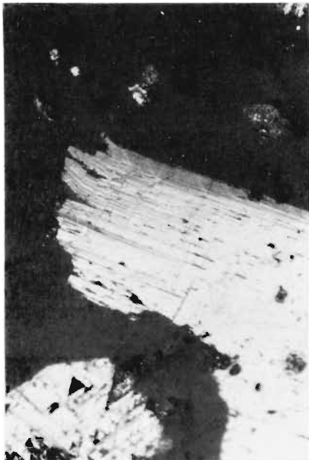
Figure 1. Polished cross section of a crystal of tungsten trioxide, reacted with potassium at 190 °C for 48 h. The width of the area shown is 10 \mu\text{m} .
